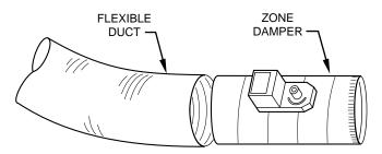
Fig 12—Round Flexible Duct Work A95132
